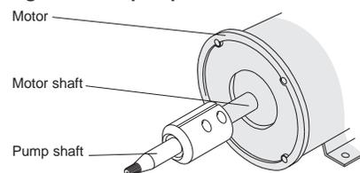
1. Lock Out power supply then disconnect the pump and motor from system.
