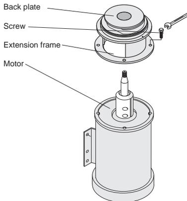
**Fig. 9: Loosen screws**
