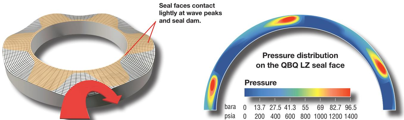
*Process fluid enters the wave valley, fluid is pressurized at the wave peaks, vapor is driven back into a liquid state, and fluid recirculates back into the seal chamber.*
