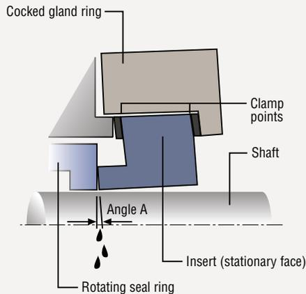
With Flowserve's flexibly mounted insert, the gland ring can be cocked and the insert remains square with the axis of the shaft.
