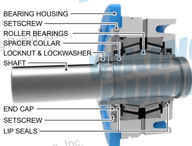
**Q, QS, M, N, R, RS Sizes:** Pack tapered roller bearings with grease and press or push bearings into housing with large end of inner races together. It is possible to install bearings incorrectly. For proper assembly see **"Figure 13"** on page 8.
