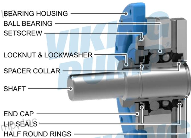
**FIGURE 13: BEARING HOUSING ASSEMBLY (Q, QS, M, N, R, RS)**
