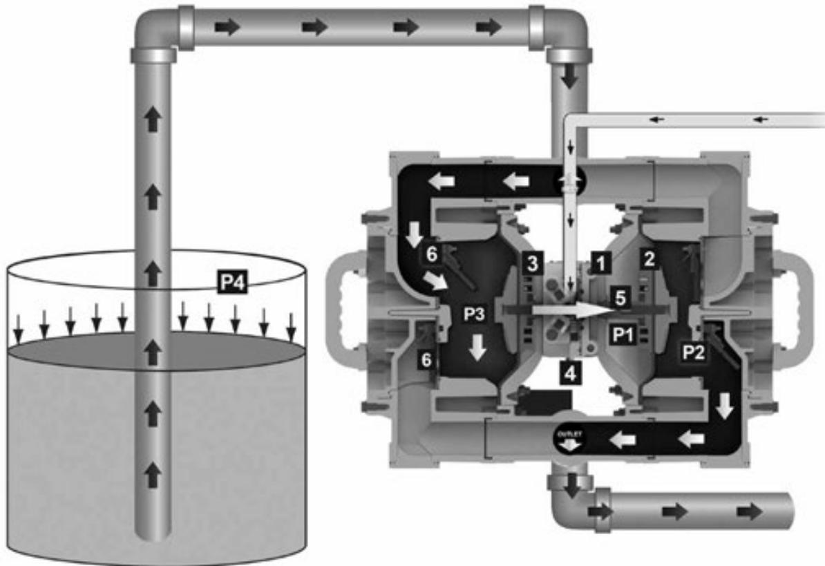
Air-Operated Double Diaphragm (AODD) pumps are powered by compressed air or nitrogen.
