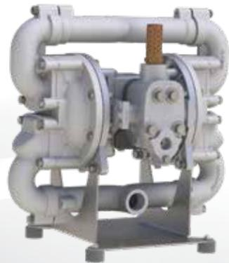
**SOLIDS HANDLING** Up to 1" (25.4 mm)    **MAX FLOW** 70 GPM (265 LPM)    **MAX PRESSURE** 125 psi (8.6 bar)    **DISPLACEMENT** 0.10 gallon (.37 liter)
