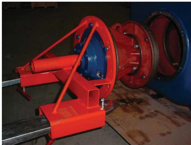
Remove your SNO8 and SNO10 powerend quickly and safely with our **SUMMIT PUMP Inc.** Powerend Removal Fixture.
