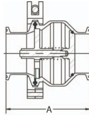
**O-ring seat with light spring (1.4 psi opening force) for low flow resistance.**
