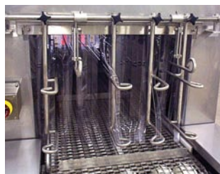
Allows multiple lane operation and adjustability for a variety of sizes while guiding totes securely
