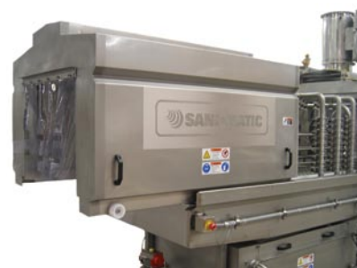
Rollaway cover provides easy access for inspection and maintenance
