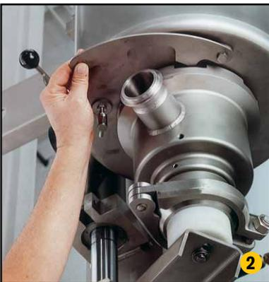
**2** Boltless V-Lock heads let you remove the shaft for inspection or routine maintenance in minutes.
