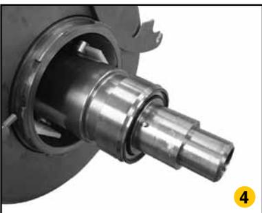
**6** The heat transfer tube is bolted to the jacket assembly. The seal design for both ends features double O-Rings. The tube can be removed easily without disturbing or disconnecting the media piping.
