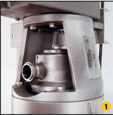
**1** After any servicing or inspection, the Votator® II reassembles quickly and easily: simply insert the self-aligning spline end of the mutator shaft into the hollow shaft in the gear motor drive. There is no complex shaft coupling, no sensitive stub shaft alignment, or vulnerable drive belts to service.
