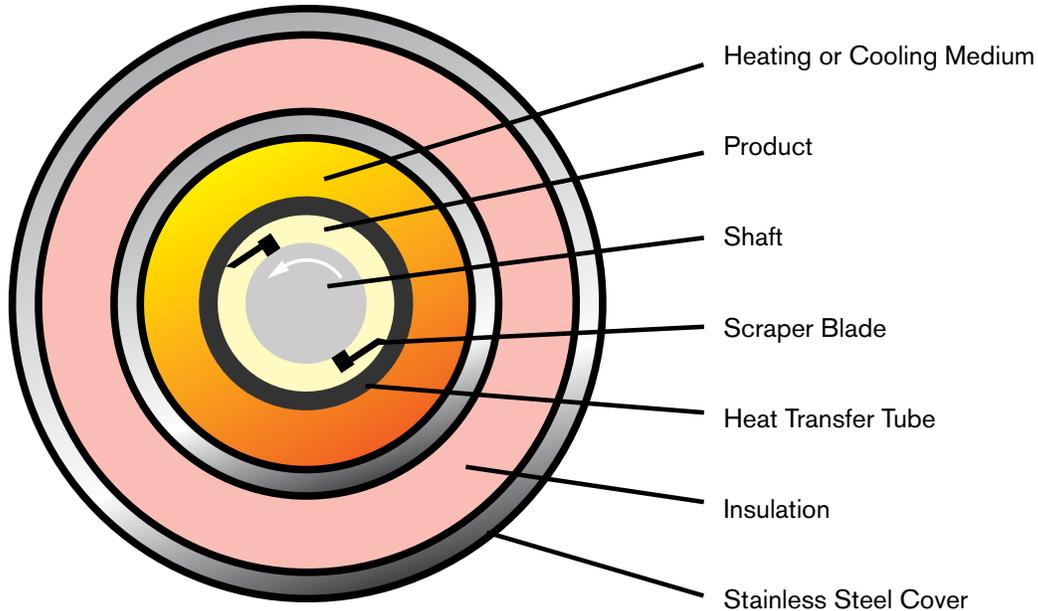
Votator's high efficiency and productivity results from a simple concept, heat or cool continuously moving product by providing a large heat transfer surface for a small amount of product in a confined space.
